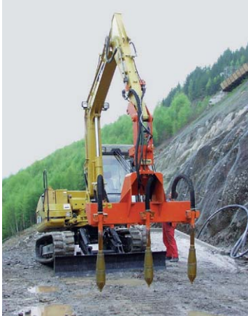
Excavator equipped with hydraulic internal vibrators from the NHR series, for compacting bulk concrete
