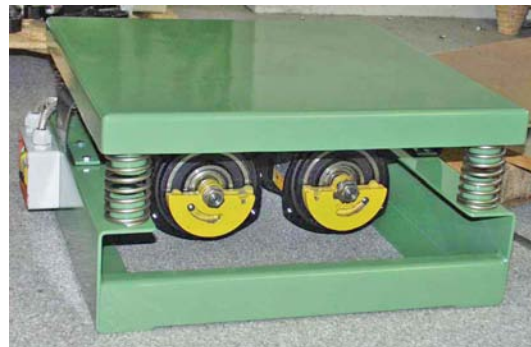
CC unbalances on 2 NEG's at vibrating table Coil springs made of stainless steel
