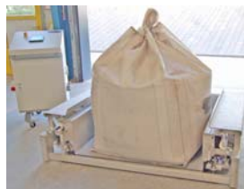
Integrated weighing system
