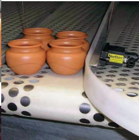
Loosening product compaction with pneumatic circular oscillators
