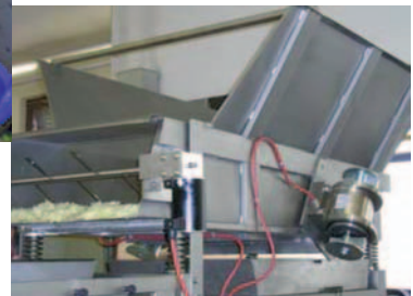
Conveying with stainless steel electric external vibrators
