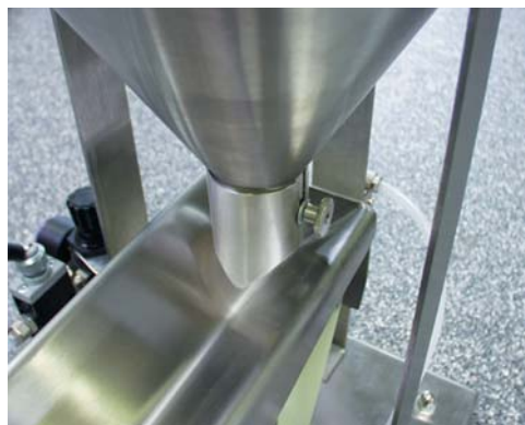
Dosing port at the silo outlet
