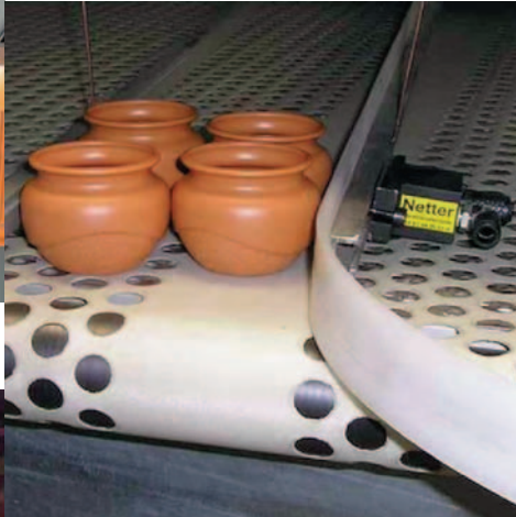
Loosening product compaction with pneumatic circular oscillators
