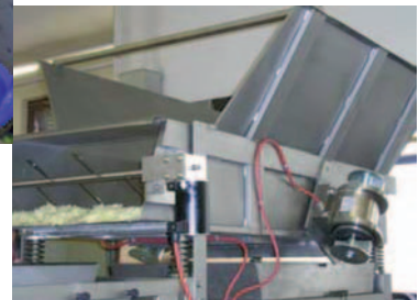
Conveying with stainless steel electric external vibrators
