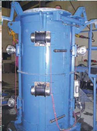
Electric external vibrators from the NEG series on a pipe form
