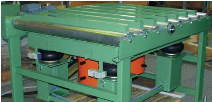
Compaction of form sand in foundry forms
