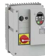
NFU frequency converters with motor output in the IP 54 housing for wall-mounting are equipped with an on-off switch, direction switch and set point potentiometer.
